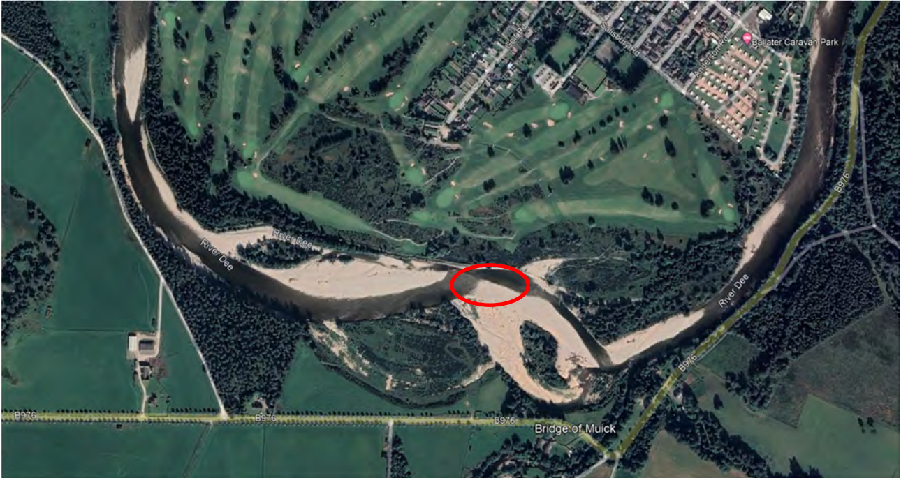
Plate 58 Google Image showing area of cobble bank that is deflecting flow towards Ballater
