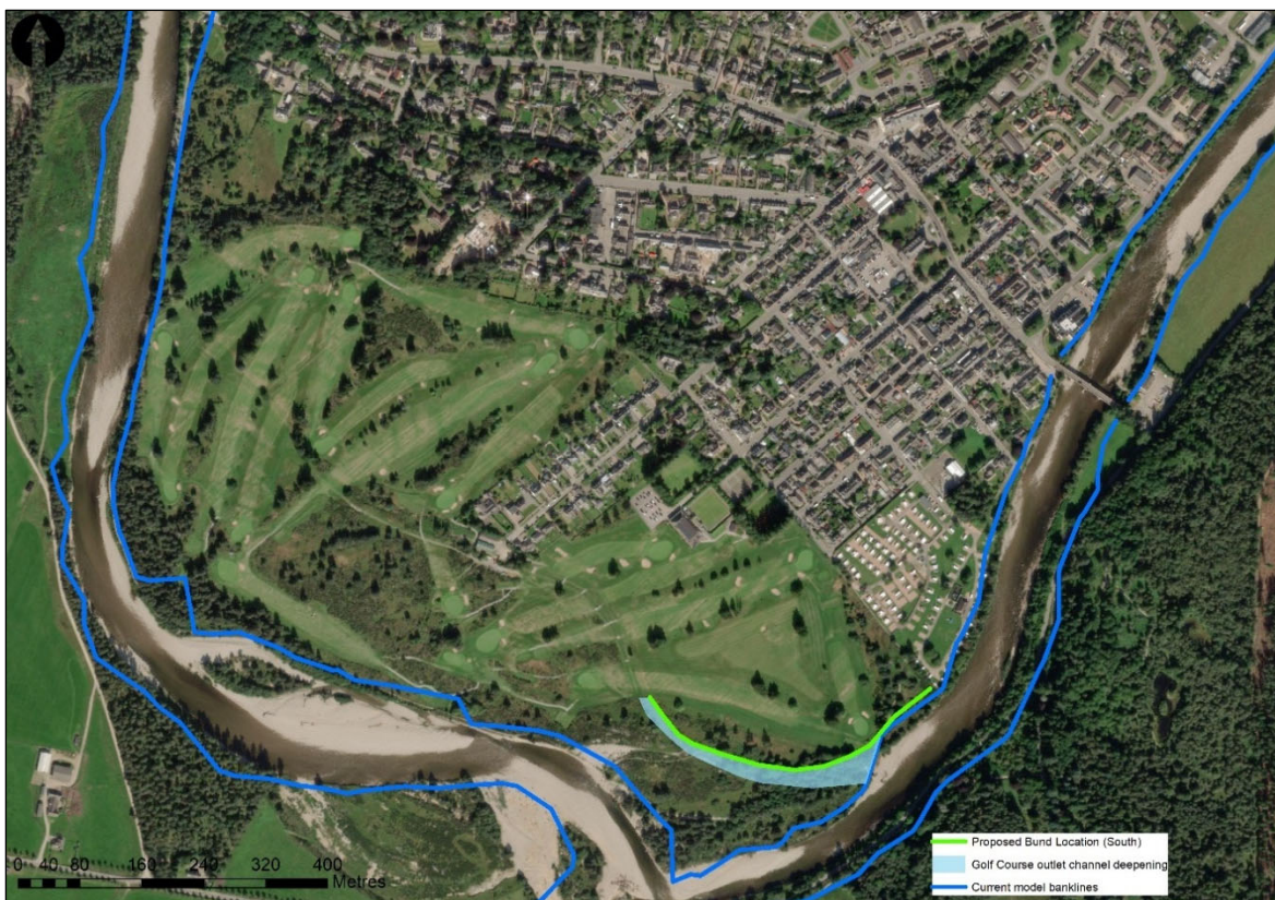
Figure 2: Option 7 South bund & clearance of outlet channel
