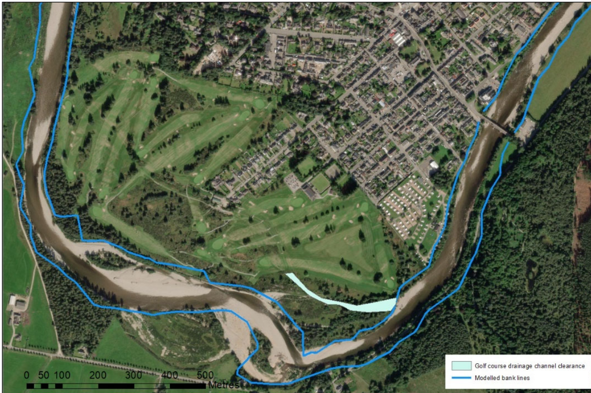
Figure 7.13: Option 3 Golf Course drainage channel clearance
