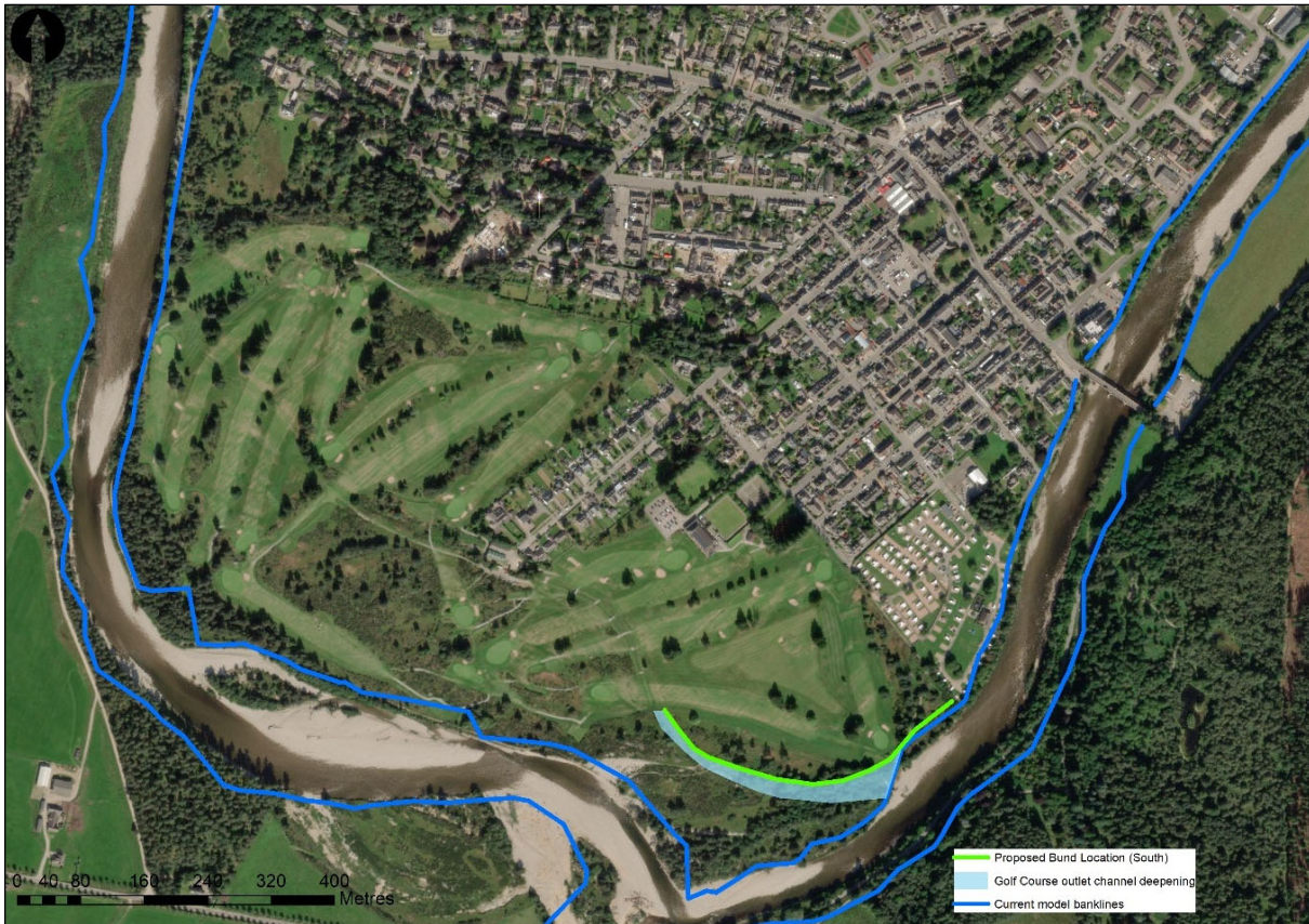
Figure 8.7: Option 7 South bund & clearance of outlet channel
